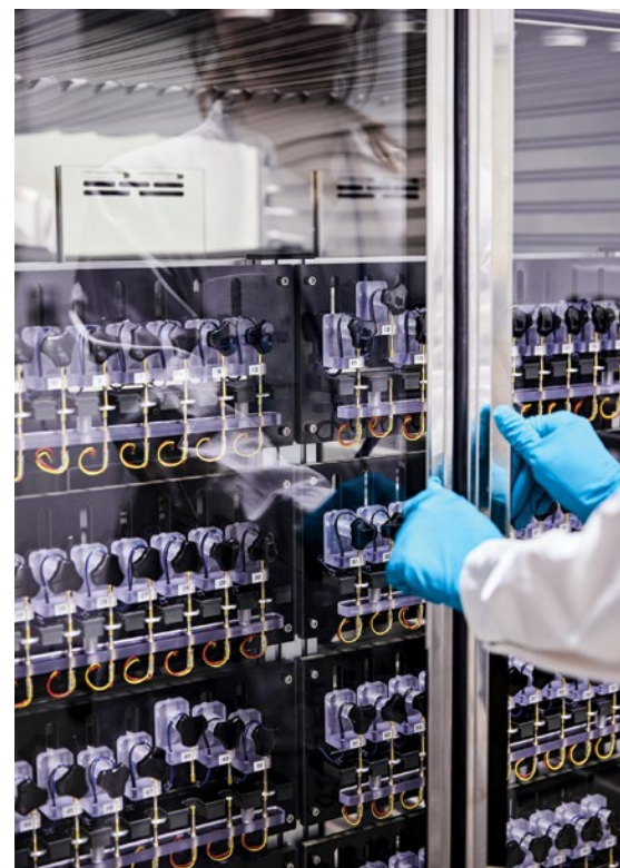
Testing coin cell batteries at Umicore
