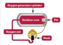
This release ignites a mixture of an oxidizer (commonly sodium chlorate) and iron powder. The heat from burning iron decomposes the oxidizer, a process that produces oxygen. The generator produces oxygen for 15-20 min, long enough for the plane to descend to an altitude at which ambient air is breathable.
