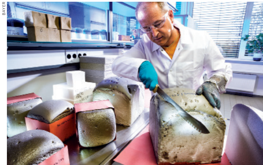
CARVE OUT A Bayer Material Science researcher prepares polyurethane samples for analysis.
