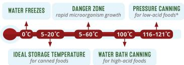
\* Pressure cooker at 10 psi (116 °C) and 15 psi (121 °C) needed to reach these temperatures
